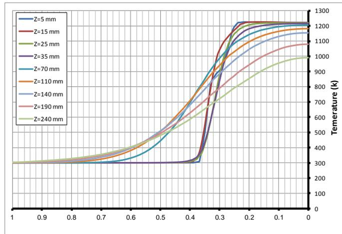
Figure (15) The temperature distribution for disk bluff body number 1 at different heights above the bluff body surface using CFD model.
