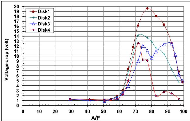
Figure (16) Effect of air to fuel ratio (A/F) on the ion current detected for Disk shape bluff body at different Blockage ratios
