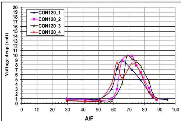
Figure (18) Effect of air to fuel ratio (A/F) on the ion current detected for cone120 bluff body at different Blockage ratios
