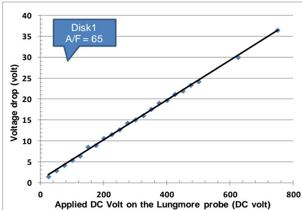
Figure (13) Impact of the applied DC volt on the voltage drop measured across the probe gap (ion current)
