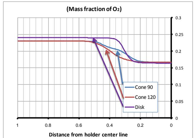
Figure (12) Some simulated output products calculated over the left half of the burner for three bluff bodies with the same blockage ratio of 0.5625 and  $V=10$  m/sec.
