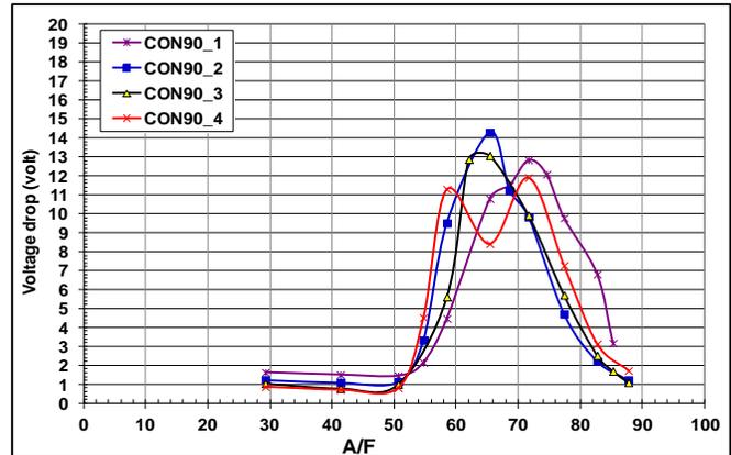
Figure (17) Effect of air to fuel ratio (A/F) on the ion current detected for cone90 bluff body at different Blockage ratios
