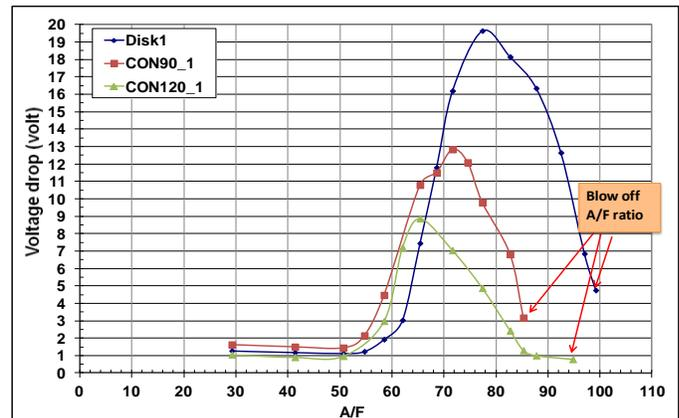
Figure (19) The voltage drop (ion current) of three bluffs body geometries with the same blockage ratio of 0.5625 and measured at 30 mm height from the bluff body surface.
