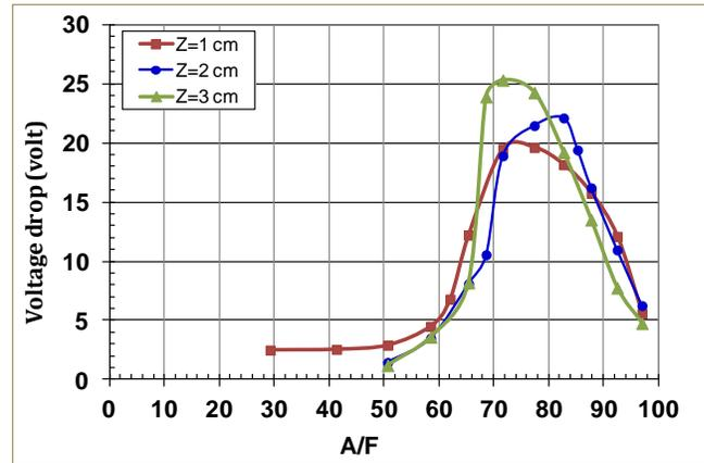
Figure (14) Voltage drop at three different heights versus A/F ratio.
