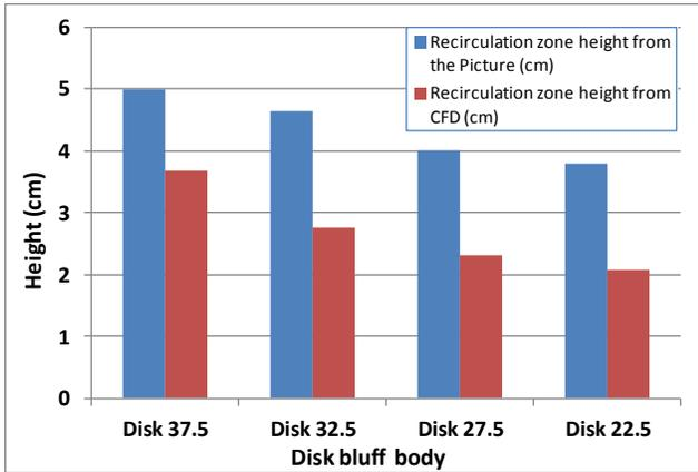
Figure (7) The recirculation zone height of four different disk bluff bodies at  $V=10$  m/s.
