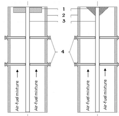
Figure (2) Test Section to show 1- Flame holder, 2- Pipe (50 mm diameter), 3- Rod (4 mm diameter), 4- Two groups of three supported bolts
