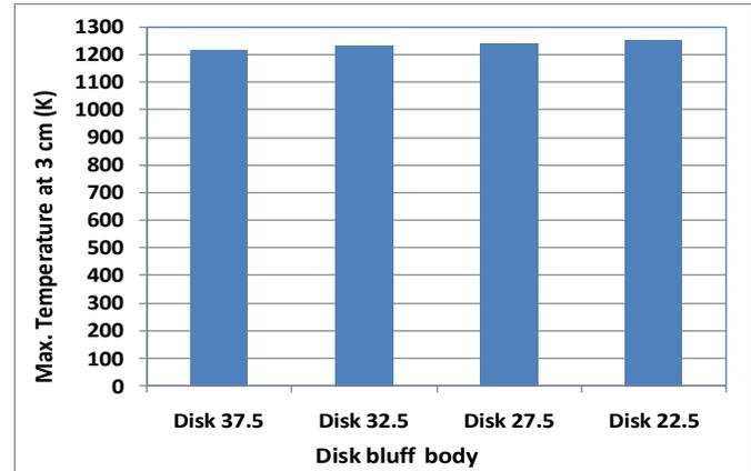
Figure (8) The maximum temperature of four different disk bluff bodies using CFD at 30 mm height from the surface and  $V=10$  m/s.
