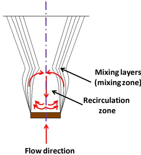
Figure (5) Schematic diagram showing the recirculation zone and the mixing zone
