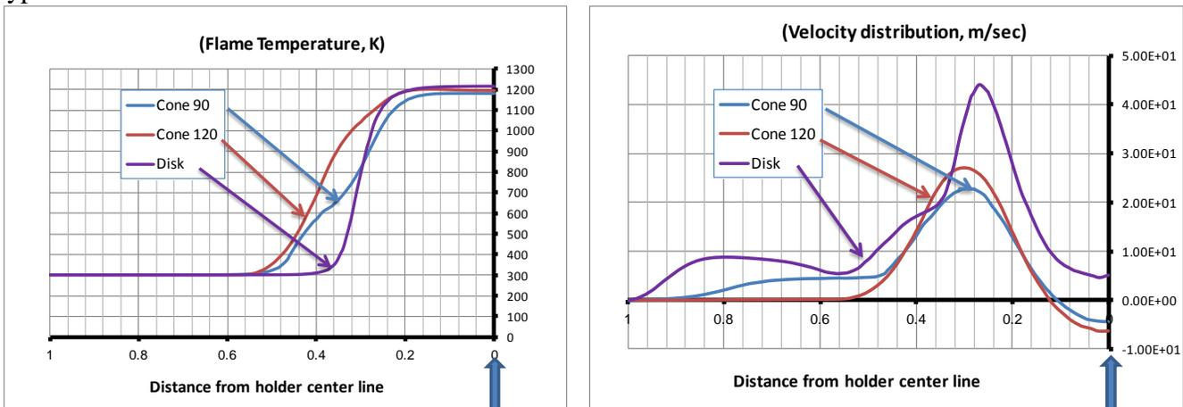
Figure (9) Simulated flame temperatures and velocity distributions over the left half of the burner for three bluff bodies with the same blockage ratio of 0.5625 and  $V=10$  m/sec.
