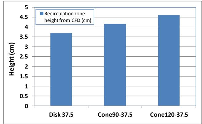
Figure (11) Recirculation zone height from CFD (cm) for three different bluff body geometries with same blockage ratio at  $V=10$  m/s
