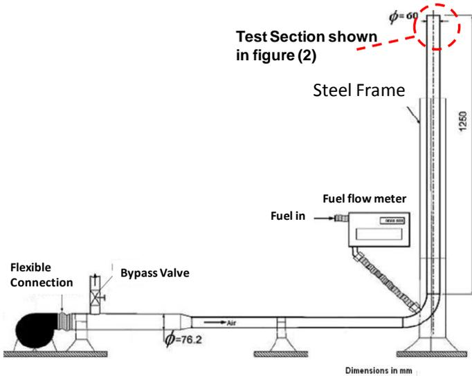
Figure (1) Layout of the experimental test rig
