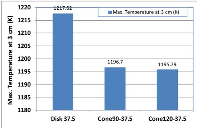
Figure (10) The maximum temperature of three different bluff body geometries measured at 30 mm height from the bluff body surface and  $V=10$  m/s.
