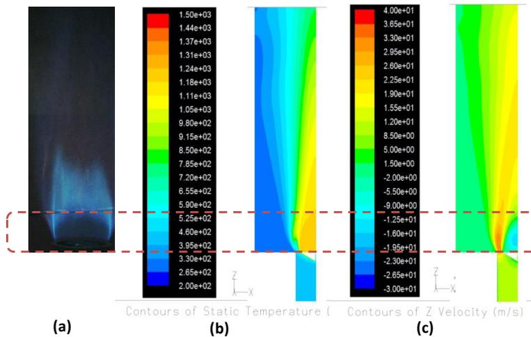
Figure (6) Comparison of (a) flame image and (b) temperature field and (c) velocity distribution calculated with CFD for Cone 120 with  $D=37.5$  mm and at  $V=10$  m/sec (dotted rectangle indicates the recirculation zone)
