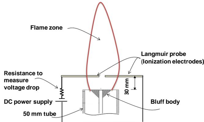
Figure (3) Langmuir probe as an ion detection method in the flame zone
